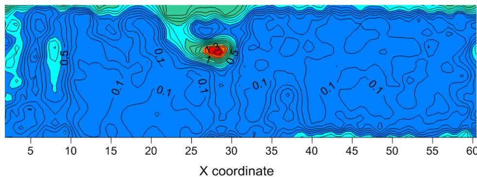
Defects of the C–C bond are observed only between atoms with a local stress value of about 1.8 GPa. One of the most stressed sections of the atomic grid containing a defect is presented in Fig. 4. From the Figure it is clearly seen that after C–C-bond breaking the atomic grid reconstructs and the stress decreases. The enthalpy of the defect formation equals  $163.5 \text{ kcal mol}^{-1}$ .
