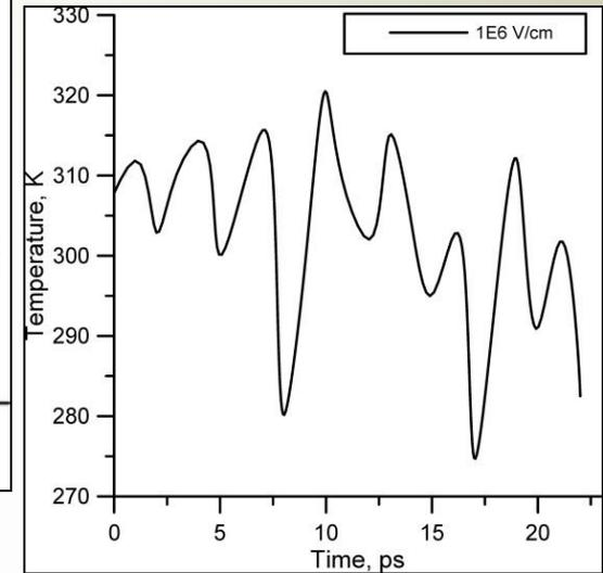
\* **C<sub>60</sub><sup>+</sup> oscillations in the potential well at  $T = 300$  K:**
