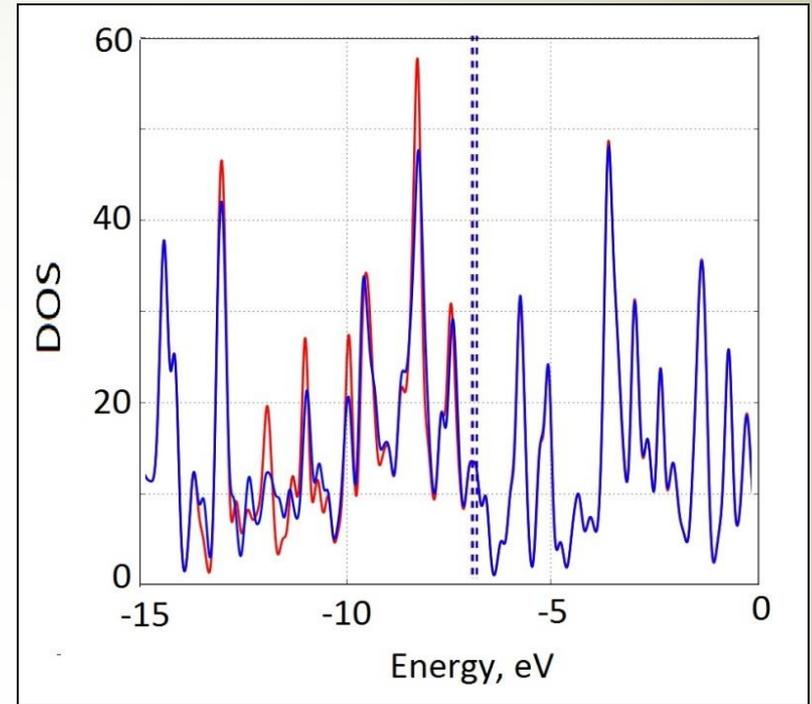
The density of electron states of complex C60+graphene near the last filled HOMO-level (vertical dotted lines indicate the position of the HOMO level).
