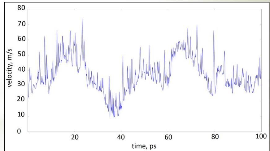
Fullerene on graphene with substrate: general view; the trajectory of the mass center at  $T = 300$  K during 100 ps; the change in the energy of interaction of C<sub>60</sub> with graphene during its free motion at  $T = 300$  K; the velocity of the fullerene C<sub>60</sub>
