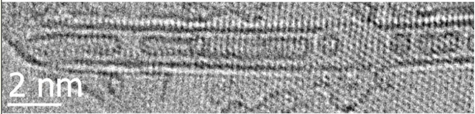
\* HR-TEM images illustrating the partial polymerization of fullerene molecules inside CNTs
