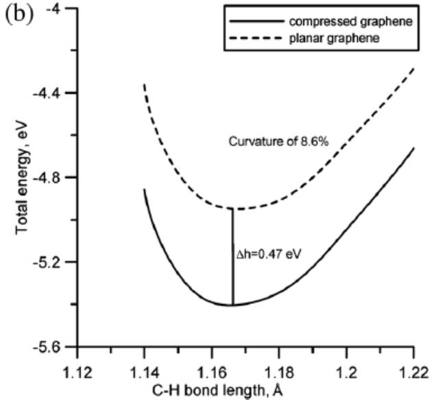
The dependence of the chemical C–H interaction energy on the length of the C–H bond for the planar and compressed graphene nanoribbon: (a) with curvature of 6.9%; (b) with curvature of 8.6%.
