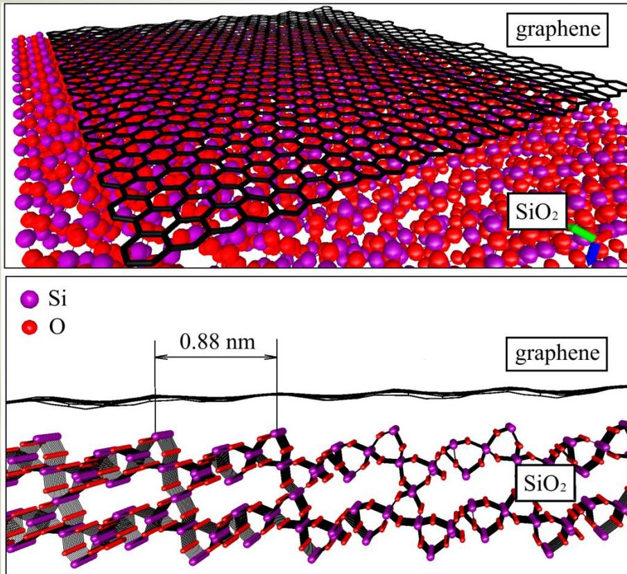
The average distance of the graphene-substrate is ~0.3 nm, the adhesion is 1.8 eV/nm<sup>2</sup> that well agrees with the experimental studies [NATURE NANOTECHNOLOGY | VOL 6 | SEPTEMBER 2011].
