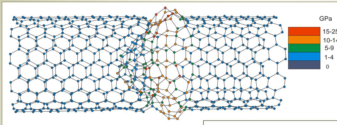
**Destruction of the structure of bamboo-like CNT during the increase of the temperature**
