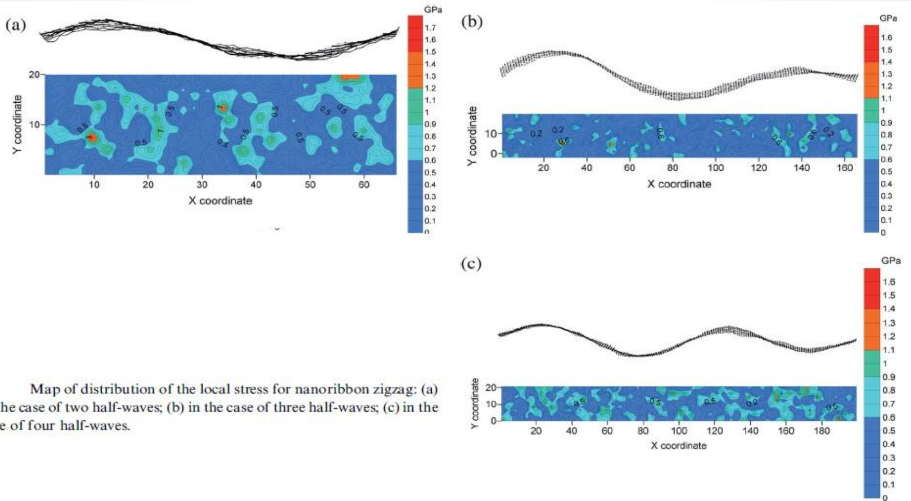
Map of distribution of the local stress for nanoribbon zigzag: (a) in the case of two half-waves; (b) in the case of three half-waves; (c) in the case of four half-waves.
